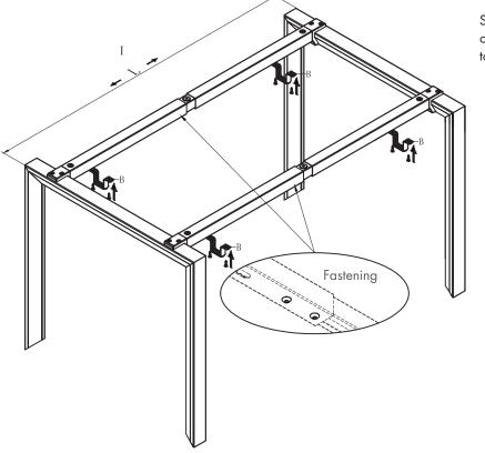
Stretch "main frame L" to the corresponding size according to the panel size.
